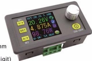
**Note:** You must make sure that input voltage is 1.1 times higher than output voltage. Under large current circumstances, pay attention to heat elimination.
